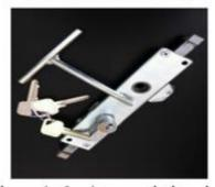
High security 3 point secure lock ready for euro barrel inserts (extra). The tongue locks the panel centrally with rods locking into the sides of the panel. 1st unlock the cylinder with a Suited (or un-Suited key), which then allows the tongue and rods to be unlocked with a Budget Lock Key.
